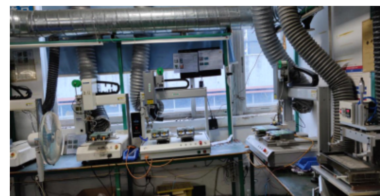
自动焊接机Automatic welding machine
